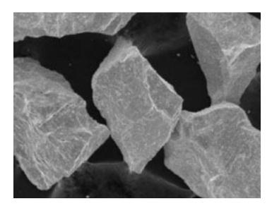
Tungcast Cast Tungsten Carbide, commonly referred to as W2C, is an extremely hard material used in a variety of applications. With a eutectic structure, high melting point and hardness, which aid in wear protection and wear resistance properties. The material is manufactured from a blend of carbon, tungsten and tungsten carbide powders and is silver / grey in colour with a sharp blocky particle shape.
